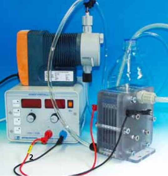
Degradation of cyanide compounds using lead-oxide and diamond electrodes in a wastewater from nickel electroplating.
